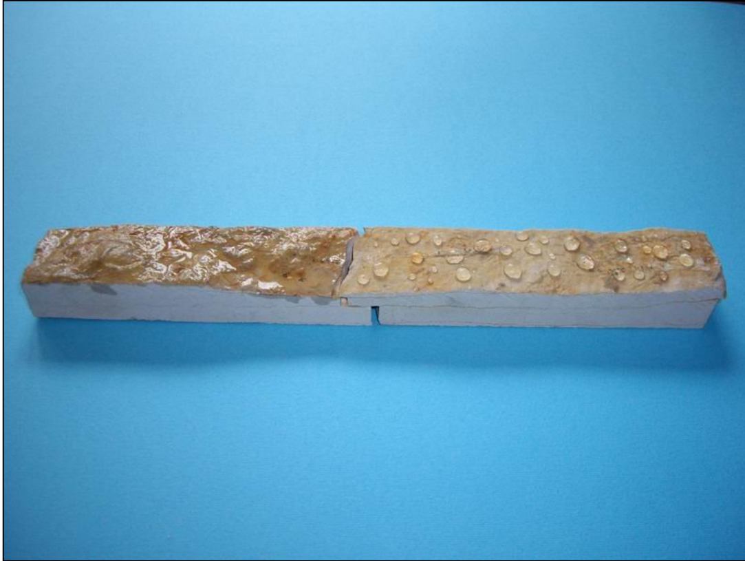
‘Struganik’ limestone: the right side is protected with Eco Impregnir K and Eco Impregnir MK , products of Development & Production Center ‘Hemi Eco’ from Belgrade
